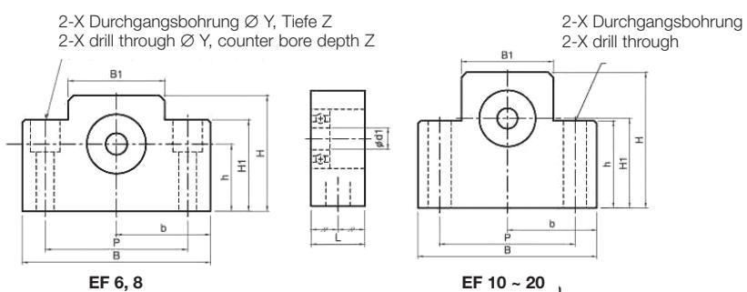
Abmessungen in mm · Dimensions in mm
