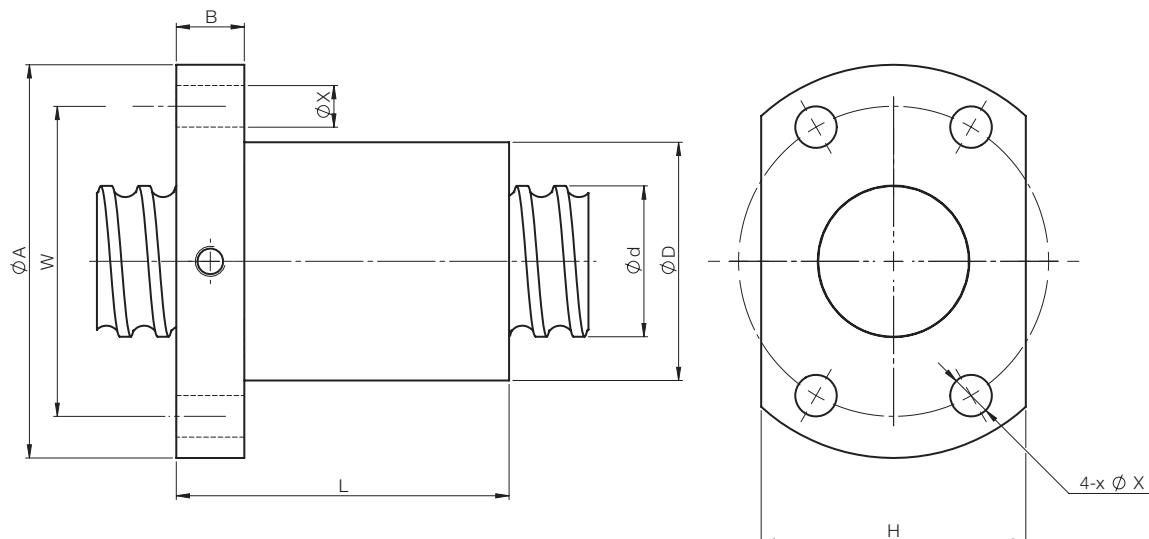
Abmessungen in mm · Dimensions in mm
