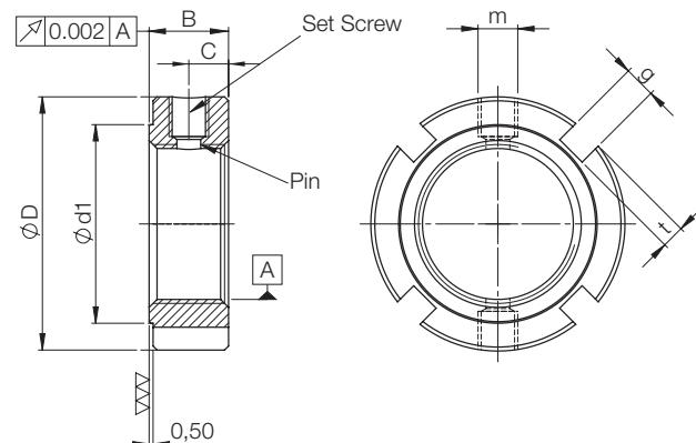
Abmessungen in mm · Dimensions in mm
